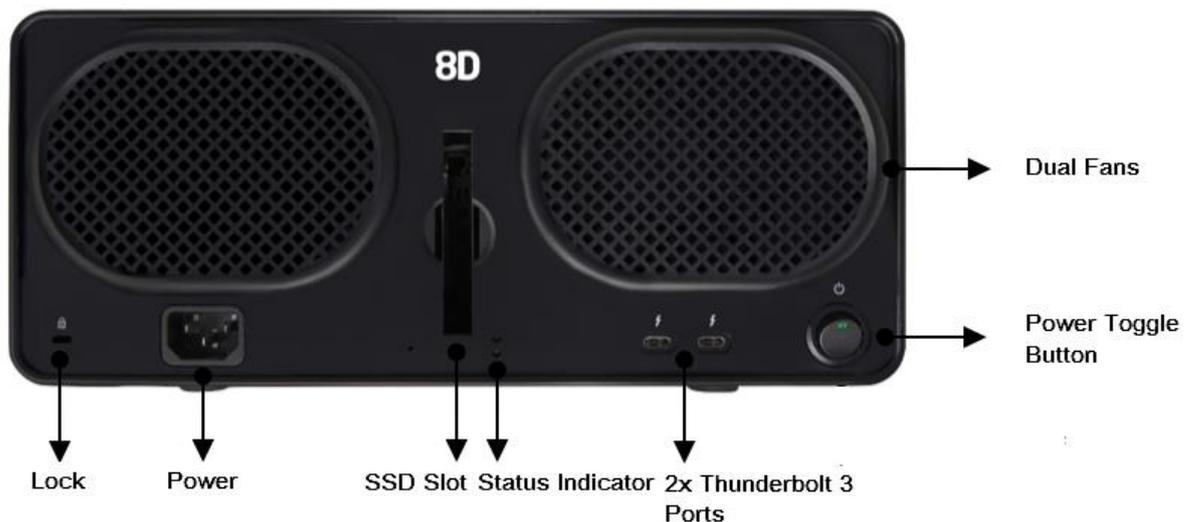
2. Slide the SSD into the back slot and gently push it down to lock in place.
