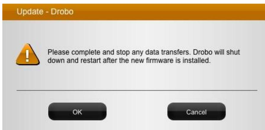
5. Ensure that the Drobo device is not actively transferring data (blinking yellow and green), and then click the **OK** button. A dialog box opens, asking you to locate the zip or TDF file on your Apple Mac™.
